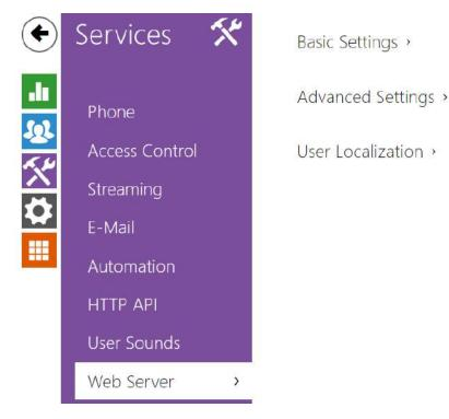
You can configure your **2N IP intercom** using a standard browser which accesses the integrated web server. Use the secured HTTPS protocol for communication between the browser and intercom. Having accessed the intercom, enter the login name and password. The default login name and password are **admin** and **2n** respectively. We recommend you to change the default password as soon as possible.
