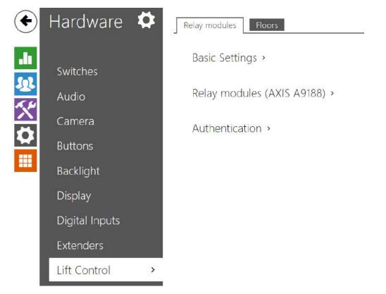
To control the floor lift access, connect the AXIS A9188 relay module to the 2N IP intercom (**2N IP Style, 2N IP Verso**, **2N IP Force**, **2N IP Safety**, **2N IP Vario**). Up to 8 relay modules can be connected to one 2N IP intercom, each of which can control up to 8 floors, which makes a total of 64.
