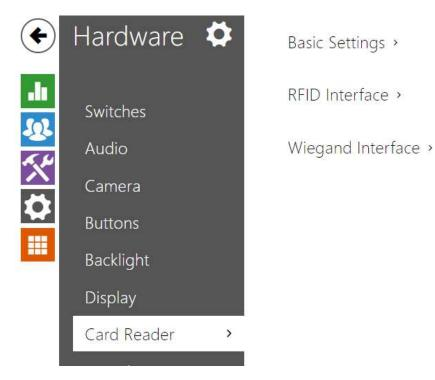
This menu is available in the **2N IP Base**, **2N IP Vario** and **2N IP Force** models only. For **2N IP Verso** only the option to limit unsuccessful access attempts is configured here. Other card reader options can be configured in the **Extenders** menu.
