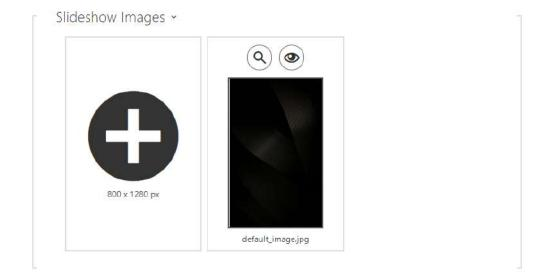
The recommended resolution is 800 x 1280 px for images in **2N IP Style**. The device automatically adjusts images with a different resolution value. Video files must have the maximum resolution of 400 x 640 px, maximum size of 7 MB and maximum framerate of 24 fps. If no image is loaded, the Slideshow mode will never be activated.
