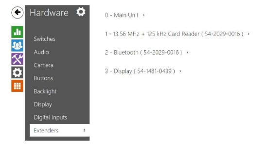
The **2N IP Verso** and **2N IP Style** intercoms can be extended by means of extending modules connected to the intercom basic unit via a VBUS. The following modules are available:
