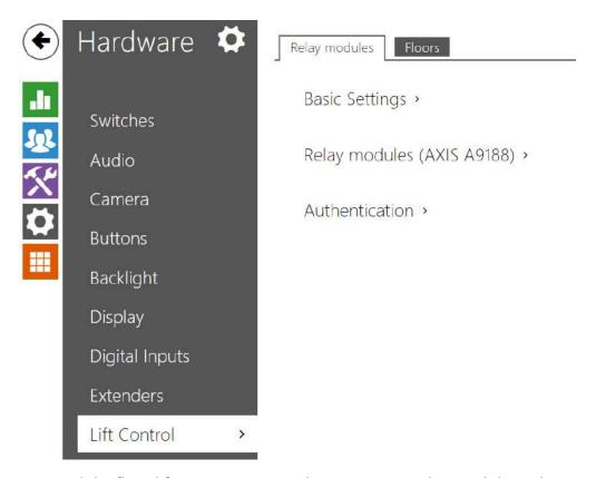
To control the floor lift access, connect the AXIS A9188 relay module to the 2N IP intercom (**2N IP Style, 2N IP Verso**, **2N IP Force**, **2N IP Safety**, **2N IP Vario**). Up to 8 relay modules can be connected to one 2N IP intercom, each of which can control up to 8 floors, which makes a total of 64.
