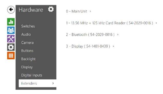
The **2N IP Verso** and **2N IP Style** intercoms can be extended by means of extending modules connected to the intercom basic unit via a VBUS. The following modules are available:
