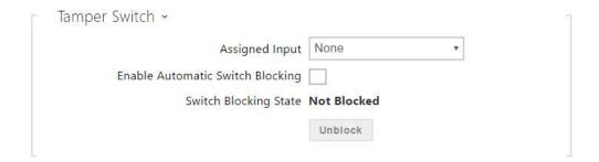
The tamper switch equipped models help detect opening of the device cover and signal this event as **TamperSwitchActivated**. The events are written into a log and read out via HTTP API (refer to the HTTP API manual).
