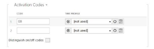
The table above includes a list of universal codes that help you activate switches from **2N Access Unit** keypad. Up to 10 universal codes can be defined for each switch (depending on the particular intercom model).
