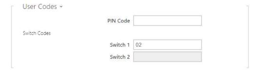
Each user can be assigned a private switch activation code. The user switch codes can be arbitrarily combined with the universal switch codes defined in the **Hardware | Switches** menu.
