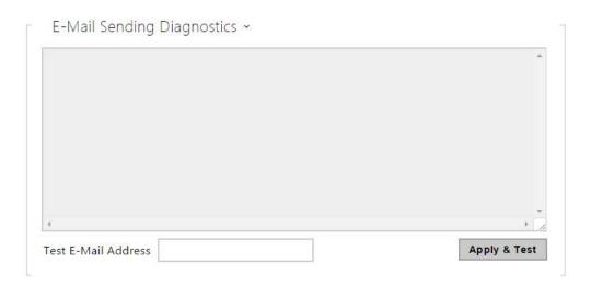
Click **Apply & Test** to send a testing e-mail to the defined address with the aim to test the functionality of the current e-mail sending setting. Enter the destination e-mail address into the Test e-mail address field and press the button. The current e-mail sending state is continuously displayed in the window for you to detect an e-mail setting problem if any on the intercom or another network element.
