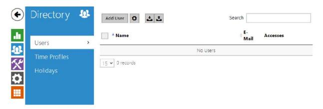
The Users list is one of the crucial parts of the intercom configuration. It contains user information relevant for such intercom functions as quick dialling, RFID card/code door unlocking, missed call e-mails and so on.
