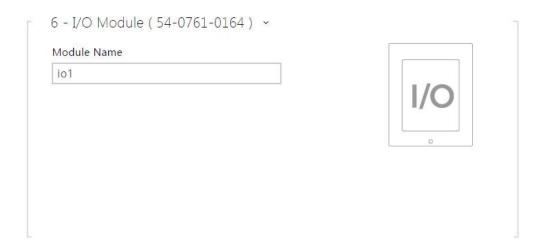
Module Name – set the module name for input/output specification in the SetOutput, GetInput and InputChanged objects in Automation.
