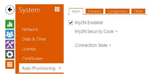
The **2N Access Unit** allows you to update firmware and configuration manually or automatically from a storage on a TFTP/HTTP server selected by you according to predefined rules.
