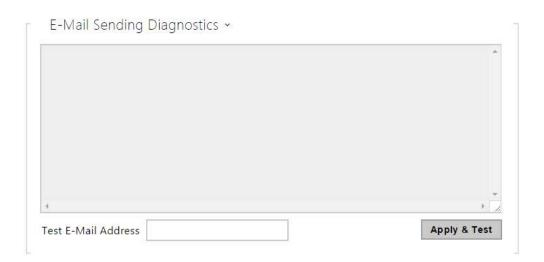
Click **Apply & Test** to send a testing e-mail to the defined address with the aim to test the functionality of the current e-mail sending setting. Enter the destination e-mail address into the Test e-mail address field and press the button. The current e-mail sending state is continuously displayed in the window for you to detect an e-mail setting problem if any on the device or another network element.
