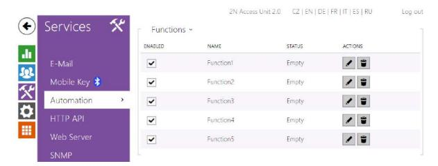
The 2N access control units provides highly flexible setting options to satisfy variable user needs. There are situations in which the standard configuration settings (switch or call modes, e.g.) are insufficient and so the device offers a special programmable interface, **2N Automation**. Typically, **2N Automation** is used in applications that require complex interconnections with third party systems.
