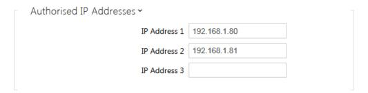
• **IP Address 1** – set IP address from which you can log in to the RTSP server. If the field is blank, any IP address can be used for login.
