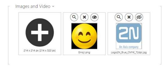
Make sure that the image resolution is 214 x 214 pixels. Other sizes will be adjusted to the display resolution automatically.
