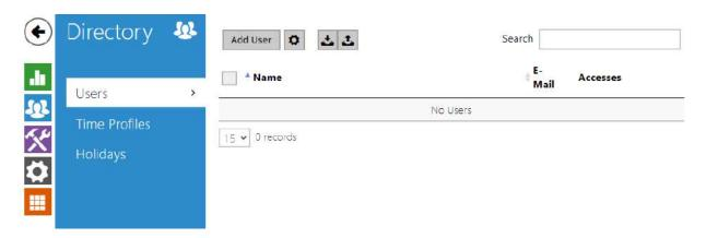
The Users list is one of the crucial parts of the device configuration. The User list contains important information about users that enables device functions such as opening doors with RFID cards, activating a combination lock, informing the user about access via email and so on. The User list contains up to 10 000 users – typically, each user is assigned just one position. The User list provides information on the users that are granted access to the building via the RFID cards.
