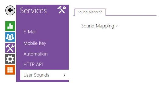
User Sounds helps you set or mute the acoustic signalling of the activated switch. For acoustic signalling for authentication refer to 5.4.1 Access Control.
