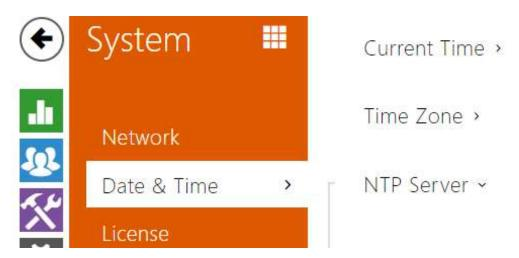
If you control validity of lock activation codes and similar by time profiles, make sure that the 2N device internal date and time are set correctly.
