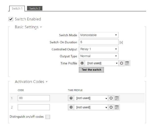
Enable the switch in the Switch Enabled parameter on the **Hardware > Switches > Switch 1** tab, set the Controlled Output to the device output to which the electric door lock is connected. Now set one or more activation codes for the electric door lock switching.
