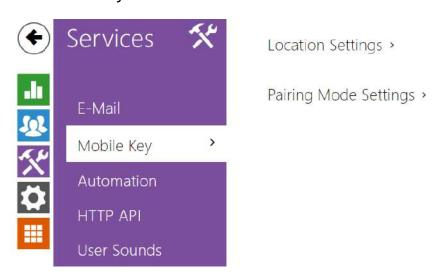
The access control units 2N can be equipped with the Bluetooth module that allows for user authentication via the **2N Mobile Key** application available to devices with iOS 12 and higher (iPhone 4 s and higher phones) or Android 6.0 Marshmallow and higher (Bluetooth 4.0 Smart supporting phones).
