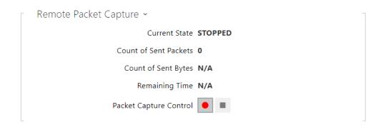
Press to start remote capturing. Specify the capturing time interval (s) for the incoming and outgoing packets. When the set time value passes, the packet capture file will be downloaded automatically to the user PC. Press to stop capturing.
