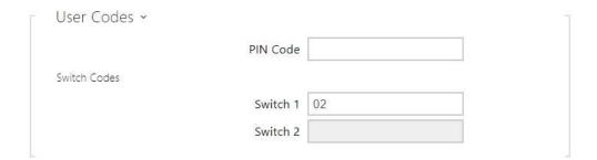
Each user can be assigned a private switch activation code. The user switch codes can be arbitrarily combined with the universal switch codes defined in the **Hardware > Switches** menu. If the codes are identical with the codes already defined in the device configuration, the mark will appear at the colliding codes.
