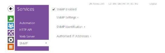
The 2N acccess control units integrate a remote device supervision functionality via the SNMP. The 2N device systems support the SNMP version 2c.
