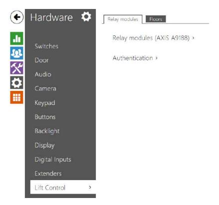
By connecting the AXIS A9188 Relay Module to the device, access to individual floors in a building can be controlled using the elevator. A maximum of 5 of these relay modules can be connected to one device, with each module controlling 8 floors, for a total of 64 floors.
