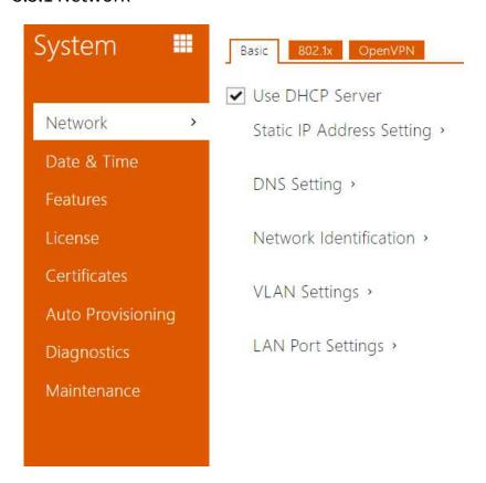
As the 2N access control units are connected to the LAN, make sure that their IP address has been set correctly or obtained from the LAN DHCP server. Configure the IP address and DHCP in the Network subsection.
