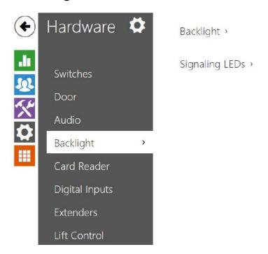
Use this tab to set the module backlight and signalling LED brightness levels separately.
