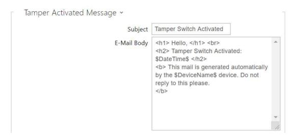
**Tamper Activated Message** – set the message to be sent to the specified e-mail address whenever the tamper switch is activated.
