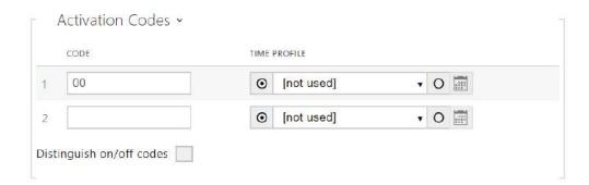
The table above includes a list of universal codes that help you activate switches from 2N device keypad. Up to 10 universal codes can be defined for each switch (depending on the particular intercom model).
