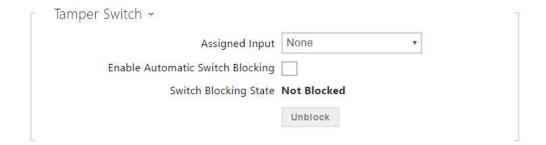
The tamper switch equipped models help detect opening of the device cover and signal this event as **TamperSwitchActivated**. The events are written into a log and read out via HTTP API (refer to the HTTP API manual).
