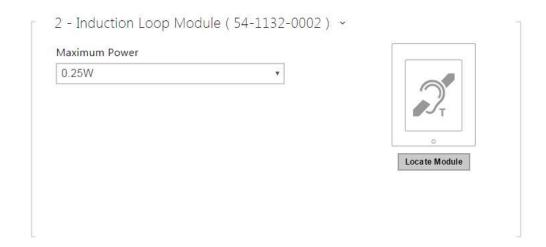
• **Maximum Power** – set the maximum transmission power for the induction loop antenna. A higher transmission power means a wider range, but less power for other functions. The convenient default value is 0.25 W under normal circumstances.
