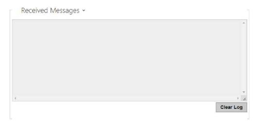
The Received Messages box helps you get the definition string. When an access card is tapped on the device reader, the counterparty's OSDP signaling definition is displayed for authorized / unauthorized access.
