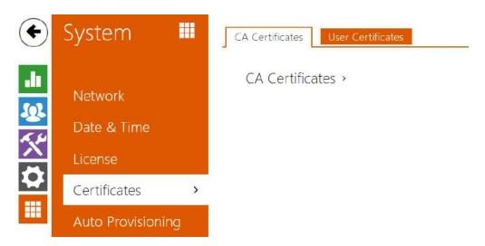
Some 2N access control units network services use the Transaction Layer Security (TLS) protocol for communication with other LAN devices to prevent third parties from monitoring and/or modifying the communication contents. Unilateral or bilateral authentication based on certificates and private keys is needed for establishing connections via TLS.
