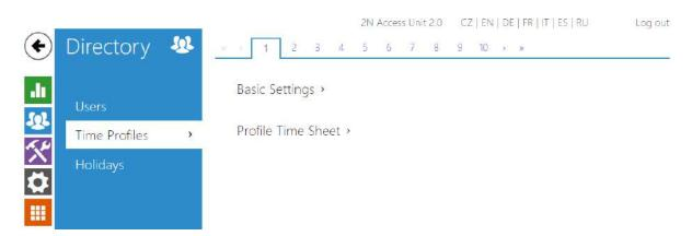
Such 2N access control units functions as RFID card/numeric code access, for example, can be time-limited by being assigned a **time profile**. By assigning a time profile you can:
