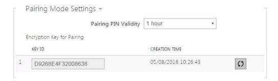
• **Pairing PIN validity** – set the authorisation PIN validity for user mobile device pairing with the 2N device.
