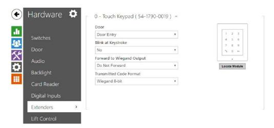
The 2N Access Unit, 2N Access Unit 2.0 and 2N Access Unit QR can be expanded using expansion modules connected via the VBUS bus. The available modules are listed in the Installation Manual of the device. Until an expansion module is connected, this section is not displayed in the web configuration interface. To view the section, it is recommended to reboot the device after connecting the expansion module.
