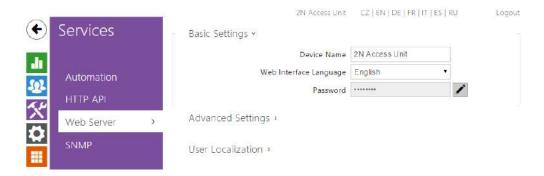
You can configure 2N access control units using a standard browser with access to the integrated web server. Use the secured HTTPS protocol for communication between the browser and 2N device. Having accessed the device, enter the login name and password. The default login name and password are **admin** a **2n** respectively. We recommend you to change the default password as soon as possible.
