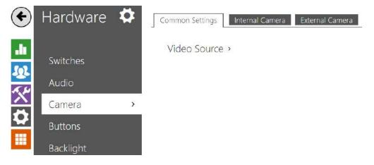
This menu is only available in the 2N device that are equipped with an internal camera or can be connected to an external camera. The camera signal can be sent by E-mail, streamed via ONVIF/ RTSP to another device (a video surveillance device, e.g.), or simply HTTP downloaded from the device in the JPEG format.
