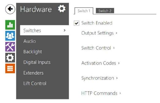
Switches provide a very flexible and efficient control of such peripherals connected to the 2N device as electric door locks, lighting, additional ringing signalling, and so on. 2N device allows you to configure to 2 independent all-purpose switches.
