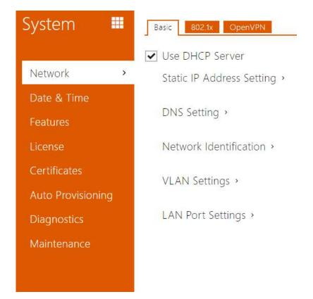
As the 2N access control units are connected to the LAN, make sure that their IP address has been set correctly or obtained from the LAN DHCP server. Configure the IP address and DHCP in the Network subsection.
