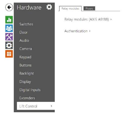
By connecting the AXIS A9188 Relay Module to the device, access to individual floors in a building can be controlled using the elevator. A maximum of 5 of these relay modules can be connected to one device, with each module controlling 8 floors, for a total of 64 floors.
