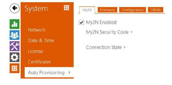
2N access control units allow you to update firmware and configuration manually or automatically from a storage on a TFTP/HTTP server selected by you according to predefined rules.
