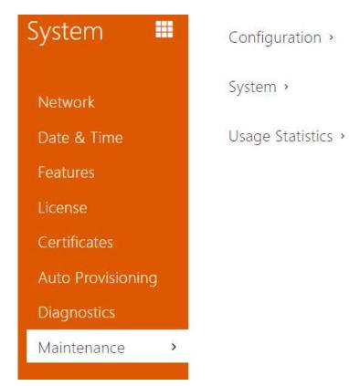
Use this menu to maintain your 2N access control units configuration and firmware. You can back up and reset all parameters, update firmware and/or reset default settings here.
