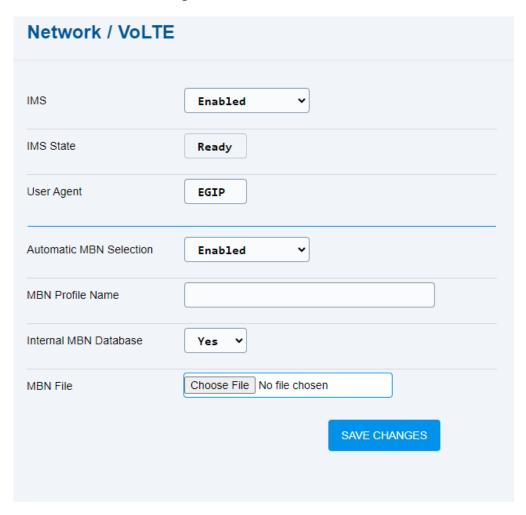
Turn on the IMS function on the Network / VolTE card to enable the VolTE function in the device. Data is enabled by the device by default, use the Network / WWAN card to change the setting. Make sure that the Network technology value on the WWAN card is always LTE (i.e. connection to LTE network) for the VoLTE calls. VoLTE calls are also available with automatic network selection if an LTE network is available.
