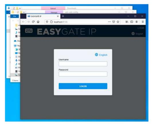
If **2N**<sup>®</sup> **EasyGate IP** is disconnected at this moment, nothing will happen. To reopen the configuration web page after USB reconnection or **2N**<sup>®</sup> **EasyGate IP** restart, for example, close and restart the 2N EasyGate IP software.
