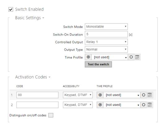
Enable the switch in the **Switch Enabled** parameter in the **Hardware / Switches / Switch 1** tab, set the **Controlled Output** to the intercom output to which the electric door lock is connected. Now set one or more activation codes for the electric door lock switching.
