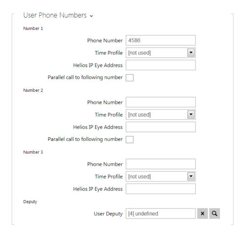
You can also use the **2N LTE intercom** with one or more IP phones without a SIP server. Use the **Direct SIP Call** for outgoing calls and enter the called phone SIP address (sip:phone\_number@phone\_ip\_address) instead of the phone number.
