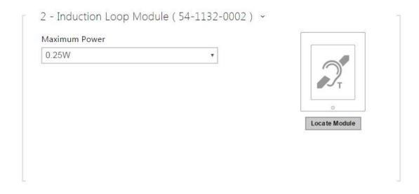
• Maximum Power – set the maximum transmission power for the induction loop antenna. A higher transmission power means a wider range, but less power for other intercom functions. The convenient default value is 0.25 W under normal circumstances.
