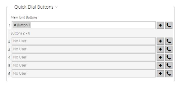
Display the list of all potentially available intercom buttons including those physically absent. In some intercom models (**2N**® **IP Vario**, **2N**® **IP Verso**), the button list is divided into 8/5-item groups corresponding to the button extending modules. Click , select the user and press Add to add a user to the editing field. To search a user in the list, use the fulltext field and the
