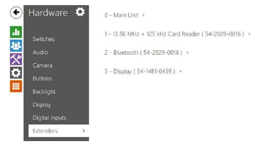
The **2N LTE Verso** intercoms can be enhanced with extending modules connected to the intercom basic unit. The following modules are available:
