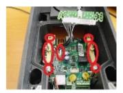
**4.** Replace 2 distance pillars from the lower side of intercom by the 2 longer distances delivered with departure switch.
