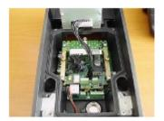
**8.** Put the keypad back. Close the intercom with top metal plate and fix it with 4 screws.
