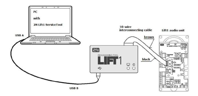
2N® Lift1 Programming Tool Connection
