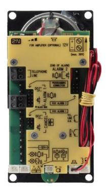
These units are installed behind the lift panel, which is prepared for installation in advance, or on the lift cabin roof.
