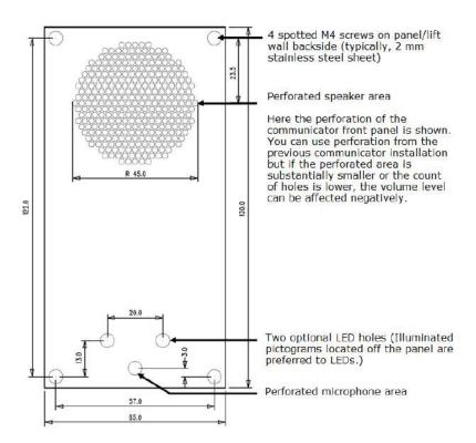
If you use other than the prescribed screws, make sure that the isolation distance between the electronics and substandard fitting elements is 2 mm at least. Make sure that the panel is fitted perfectly to avoid resonance during operation. There may be no gap between the lift button panel and **2N**<sup>®</sup> **Lift1** or the gap must be sealed properly to eliminate acoustic fault of the speaker and acoustic feedback between the speaker and microphone (see below).
