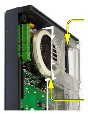
Poorly tightened screw (a squeezed wire has the same effect)
