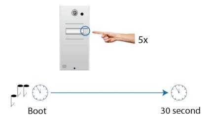
• 3-buttons models: Press the second quick dial button on the basic unit five times.
