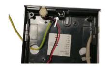
Assemble the set and ground the cable.
