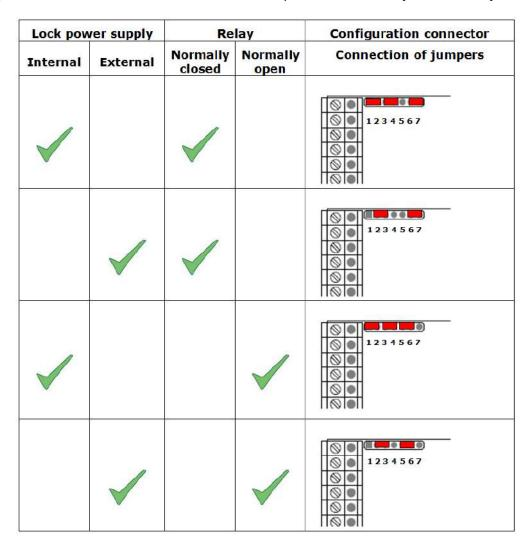
**Connection of Configuration Connector Jumpers**
