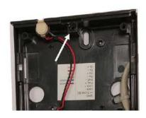
Insert the crimped cable at the marked point.
