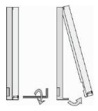
3. Use a cross-head screwdriver to remove the plastic cover and demount the cover.
