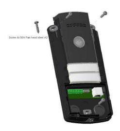
Position of Mounting Screws on 2N® IP Base
