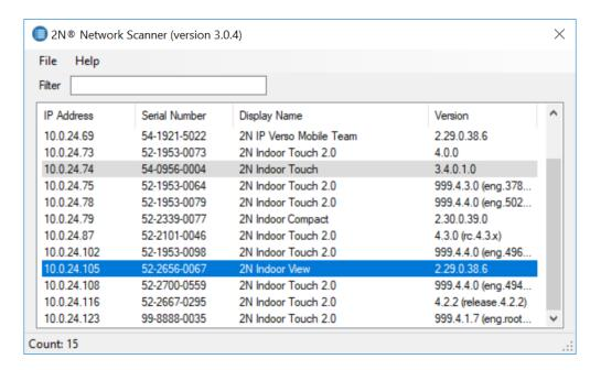
To find the **2N** \*\*Indoor View IP address using the display, press any key on the display to quit the sleep mode. The Settings menu is displayed on the home screen after pressing the settings icon in the bottom right corner. Find the IP address information in the Settings / About device menu.
