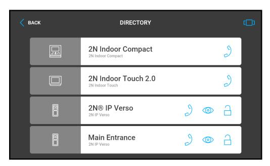
Find the Directory menu under the phone earpiece icon The menu provides a list of destinations that can be called. The destinations include their names and the device type they are equipped with. The Directory provides either a list view where you can scroll up/down, or a tile view where you can browse from right to left to choose a destination.
