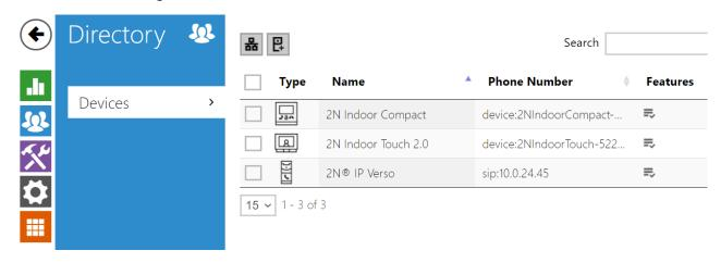
Directory is one of the crucial parts of the device configuration. It helps add new devices (2N IP intercoms and other answering units) and provides essential information on them. Up to 200 devices can be added to the directory.
