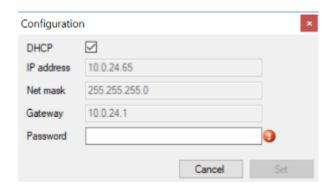
2N® IP Network Scanner IP Address Change
