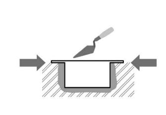
Make sure that the flush mounting box is slightly above the wall surface not aligning with the wall. A wrong installation may lead to water penetration and subsequent damage of the device. Use the side protrusions to achieve the proper flush mounting.
