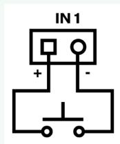
• Wiring diagram of IN1, IN2 and IN3 terminals in passive mode
