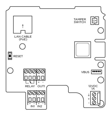
2N Access Unit Connectors, PCB Version 599v3 and 599v4
