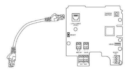
UTP Cable Connection to 2N Access Unit Terminal Board
