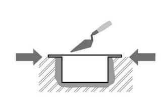
Make sure that the flush mounting box is slightly above the wall surface not aligning with the wall. A wrong installation may lead to water penetration and subsequent damage of the device. Use the side protrusions to achieve the proper flush mounting.
