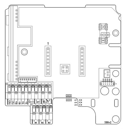
**2N Access Unit** Connectors, PCB Version 586v2
