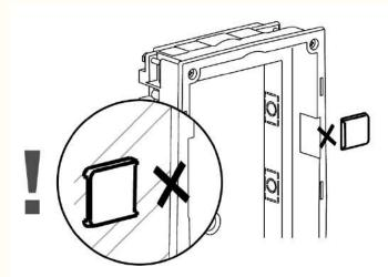
• Break off the side protrusions when the walling material has hardened.
