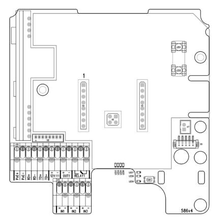
2N Access Unit Connectors, PCB Version 586v4
