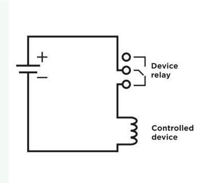
Electric circuit opening diagram for controlled devices with PCB version 586v2 and below
