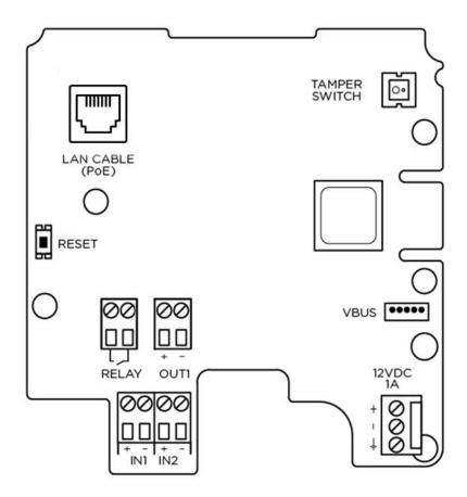
2N Access Unit 2.0 Connectors, PCB Version 599v6
