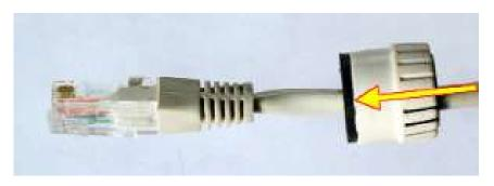
5. Pull the cable connector though the bushing body into the intercom and clip it into the motherboard connector.
