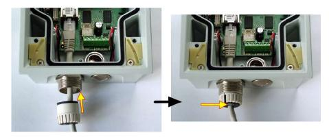
2. Remove the sealing including the cover from the bushing. Cut either of the components as shown in the figures.
