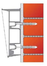
Wall (surface) mounting is used where flush mounting is inapplicable (in concrete and steel structures, entry barrier columns, etc.). The frame is not used.
