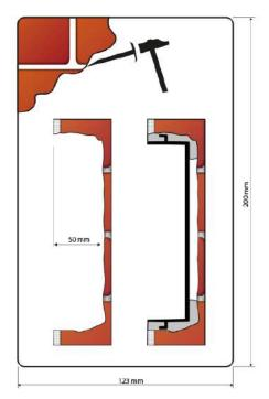
Hole dimensions for flush mounting
