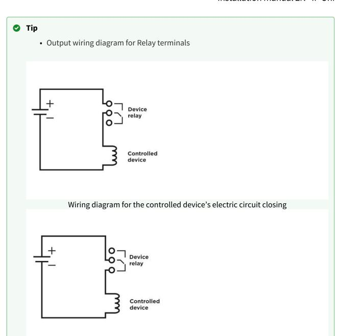
Wiring diagram for the controlled device's electric circuit opening
