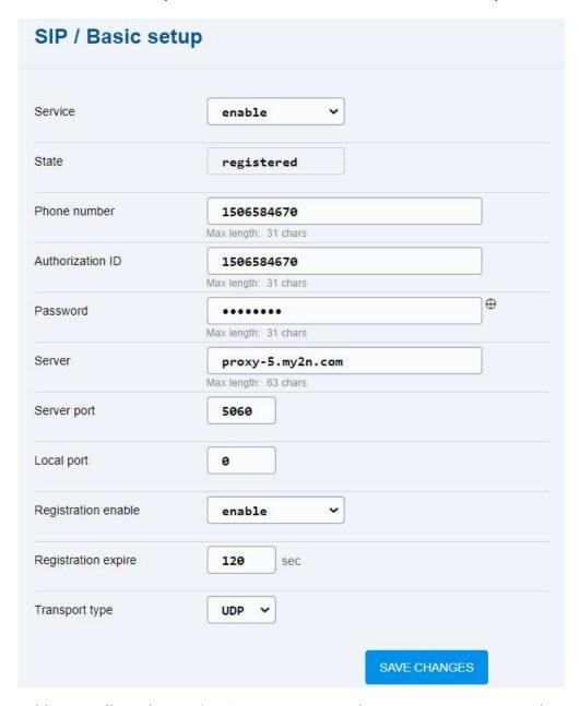
Enable SIP calls in the SIP / Basic Settings menu by turning on Service and save the setting. Complete the phone number and authorization ID if different from the phone number. Enter the password paying attention to the lower/upper case. Complete the SIP server address. If 0 is set by default, the setting is same as in 5060.
