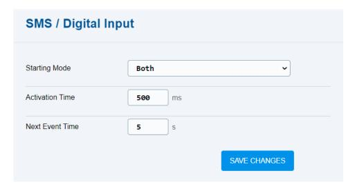
• **Starting Mode** – select the digital input change mode that triggers SMS sending.
