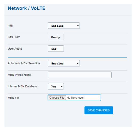
Turn on the IMS function on the Network / VolTE card to enable the VolTE function in the device. Data is enabled by the device by default, use the Network / WWAN card to change the setting. Make sure that the Network technology value on the WWAN card is always LTE (i.e. connection to LTE network) for the VoLTE calls.
