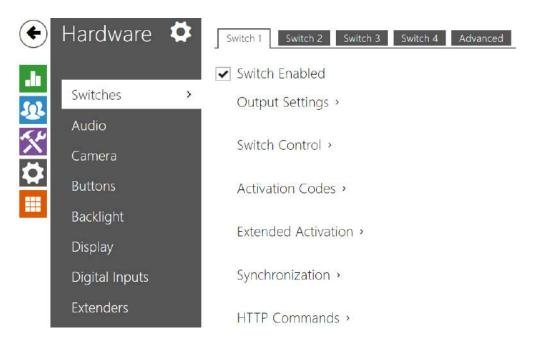
Switches provide a very flexible and efficient control of such intercom peripherals as electric door locks, lighting, additional ringing signalling, and so on. **2N LTE intercoms** allows you to configure up to 4 (depending on model types) independent all-purpose switches.
