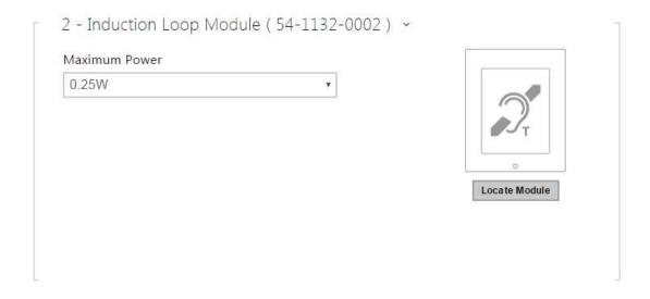
• Maximum power – set the maximum transmission power for the induction loop antenna. A higher transmission power means a wider range, but less power for other intercom functions. The convenient default value is 0.25 W under normal circumstances.
