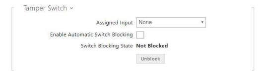
The tamper switch equipped models help detect opening of the device cover and signal this event as **TamperSwitchActivated**. The events are written into a log and read out via HTTP API (refer to the HTTP API manual).
