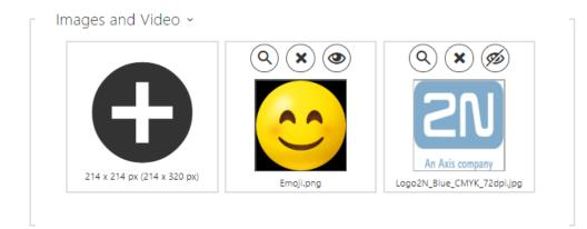
Make sure that the image / video resolution is 214 x 214 or 214 x 320 pixels up to 2 MB. Other sizes will be adjusted to the display resolution automatically.
