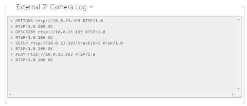
The External IP Camera Log displays the RTSP communication with the selected external IP camera including failures and error states if any.
