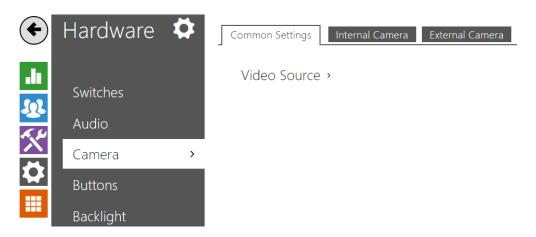
This menu is only available in the **2N IP intercom** models that are equipped with an internal camera or can be connected to an external camera. The camera signal can be streamed directly into the call via a videophone, sent by E-mail, streamed via ONVIF/RTSP to another device (a video surveillance device, e.g.), or simply HTTP downloaded from the intercom in the JPEG format.
