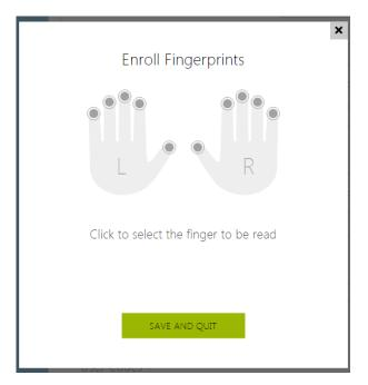
Up to two fingerprints may be saved for each user. **3)** Click SCAN FINGER to load a fingerprint.
