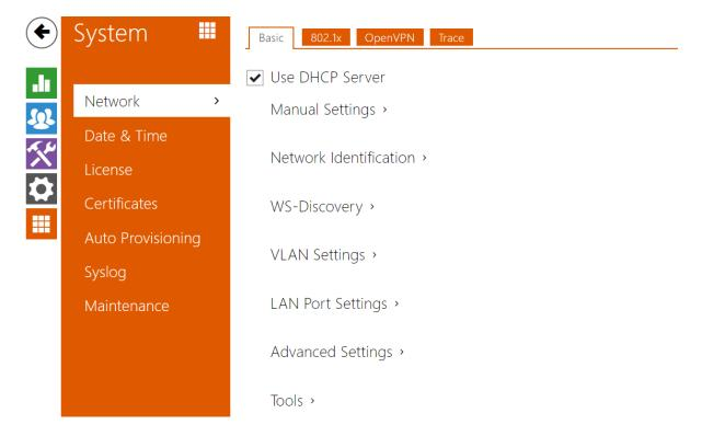
As the **2N IP intercom** is connected to the LAN, make sure that its IP address has been set correctly or obtained from the LAN DHCP server. Configure the IP address and DHCP in the **Network** subsection.
