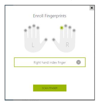
**4)** Place the selected finger on an external USB reader. This process is repeated three times for greater precision.
