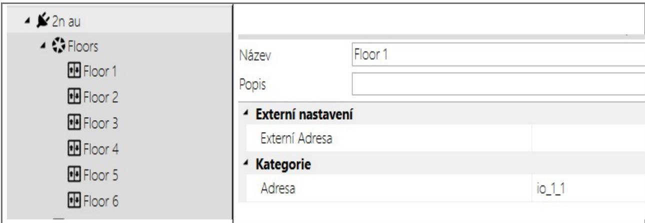
Access for individual people is then set on the individual floors. The state of the floors is always active, this is because the 2N device does not possess any information whether the attached relay modules are online.
