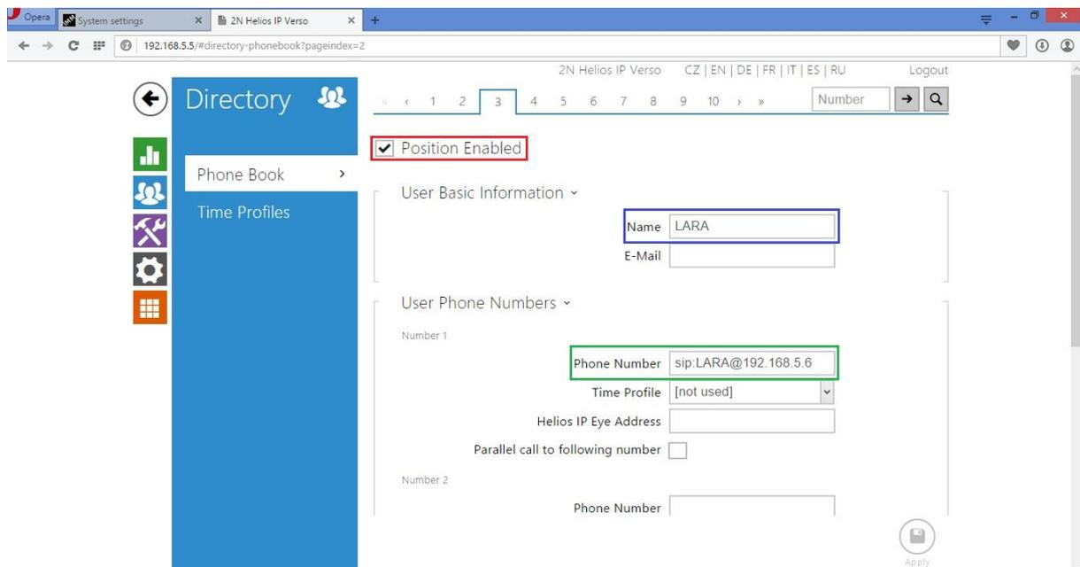
*Image: For the LARA device, not the address of the iMM server, but rather the IP address of the given LARA device, is entered with the Asterisk server*
