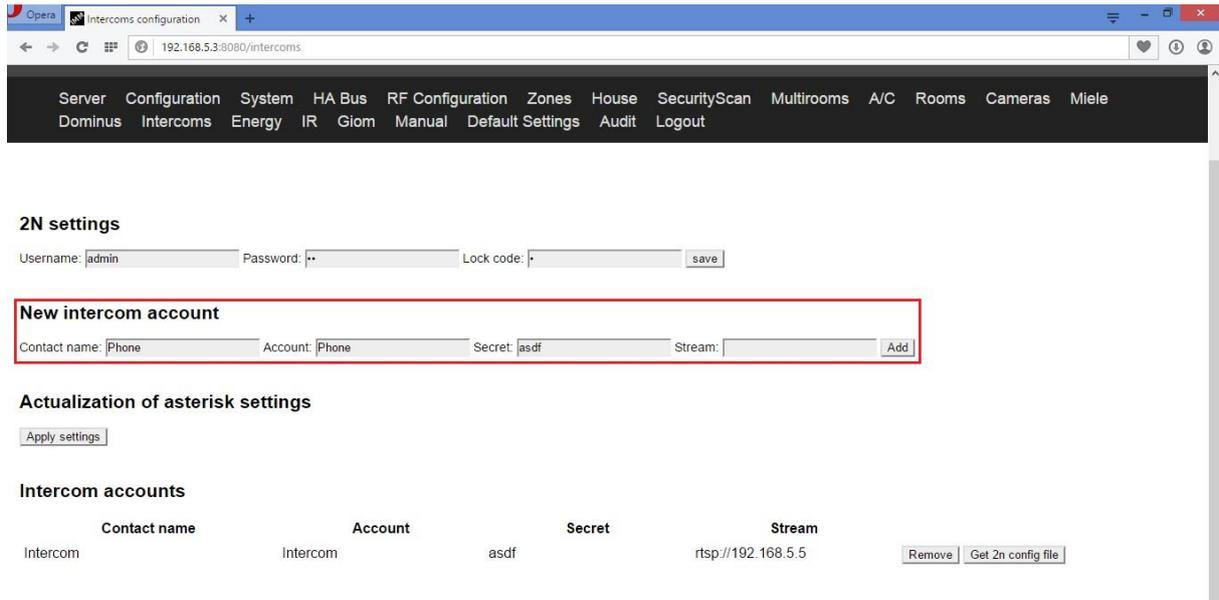
Image: Example of a created account for the iHC application in the smartphone (the stream for access to the video camera is not entered)
