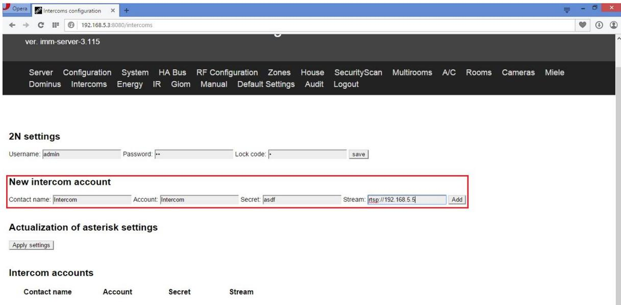
*Image: Creating an account for the intercom including entering the video camera stream*
